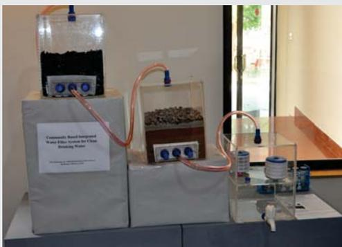
The preparation of new material for the above purpose is the main novelty in the presented work. The system is composed of material (biosand, polymers etc) that are easily available and cheap. Moreover, the designed filter contains various desired component as a single unit system i.e. appropriate pore size, porous surface roughness, interconnectivity and surface
